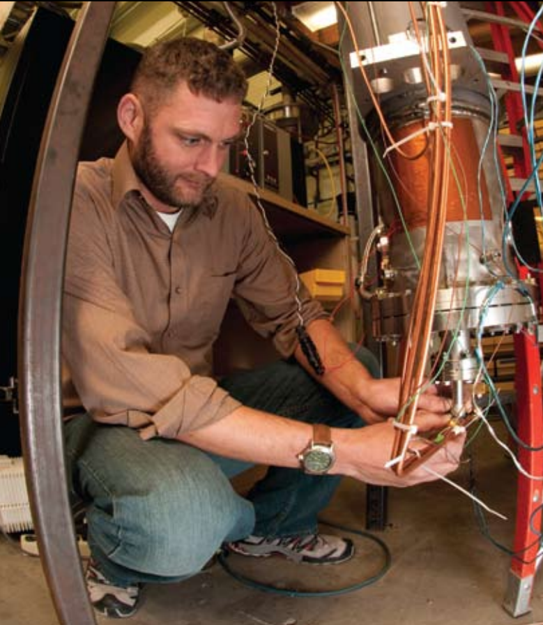
John Popielarski, engineer at the National Superconducting Cyclotron Laboratory, works on the superconducting coaxial resonator, which accelerates particles toward detectors.
