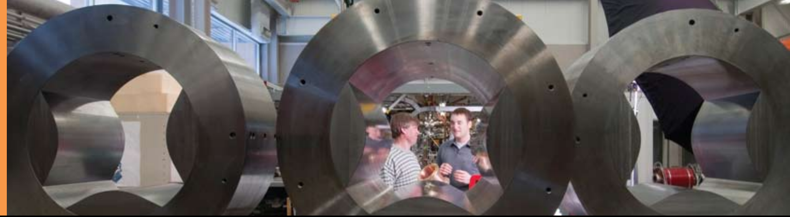
Chris Magsig (left), research and development engineer, and Philip Voss, graduate student, at the National Superconducting Cyclotron Laboratory, are seen through the A1900 quadrupole triplet—magnets that will be used for momentum compression for ReA3, the new reaccelerator.
